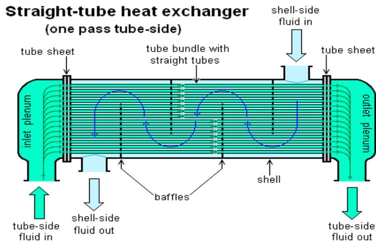
Figure 4 : Shell and Tube Heat Exchanger
