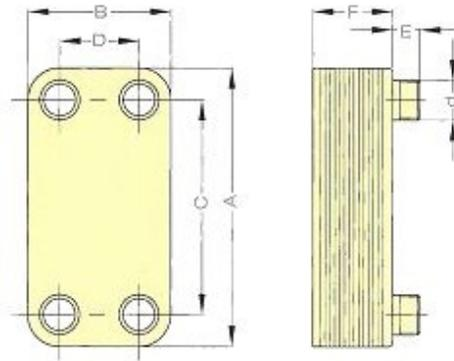
**Figure 6: Brazed Plate Heat Exchanger**
