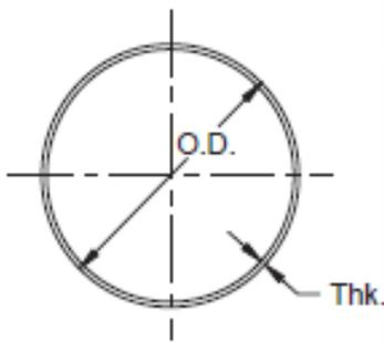
**Figure 3: Pipe diagram**
