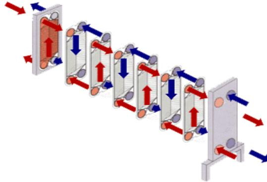
Figure 5: Plate Heat Exchanger
